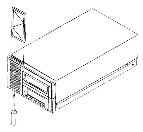
Figure 8-3. Air Filter Removal
